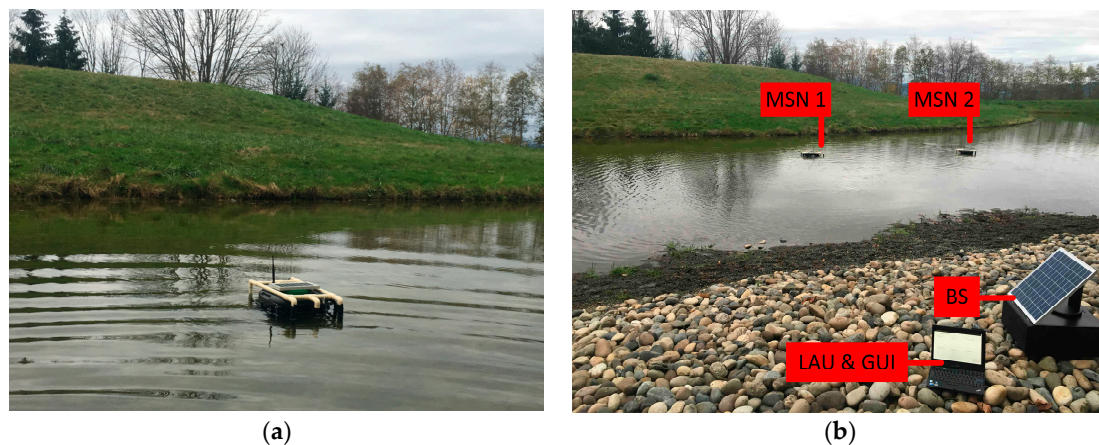
Figure 6. Field deployment of the developed platform at the Yosef Wosk Reflecting Pool: (a) Deployment of the MSN in the pool; (b) Deployment of the platform in the field.
