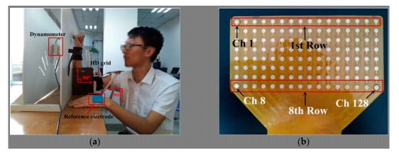
**Figure 2.** (**a**) The apparatus to aid the recording process. (**b**) The arrangement of electrodes on the HD grid.
