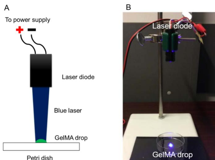
Figure 1. System setup (A) Schematic and (B) Photo of the simple laser crosslinking system
