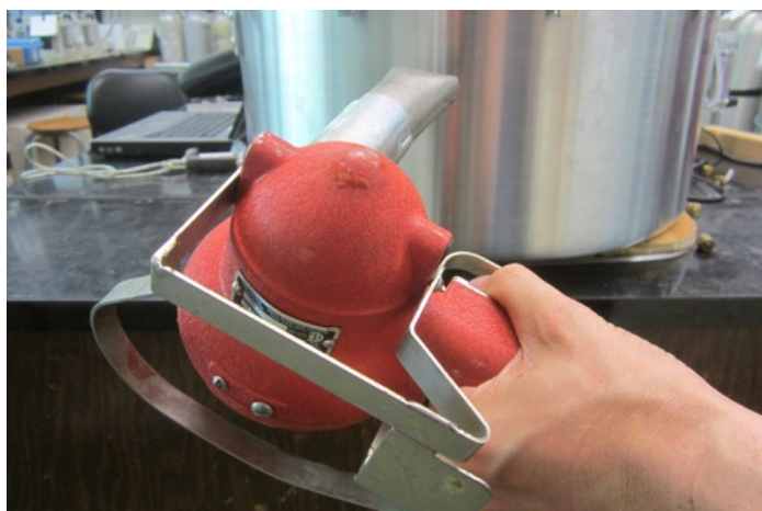
Figure 4 - Heating the container's exterior with a heat gun.
