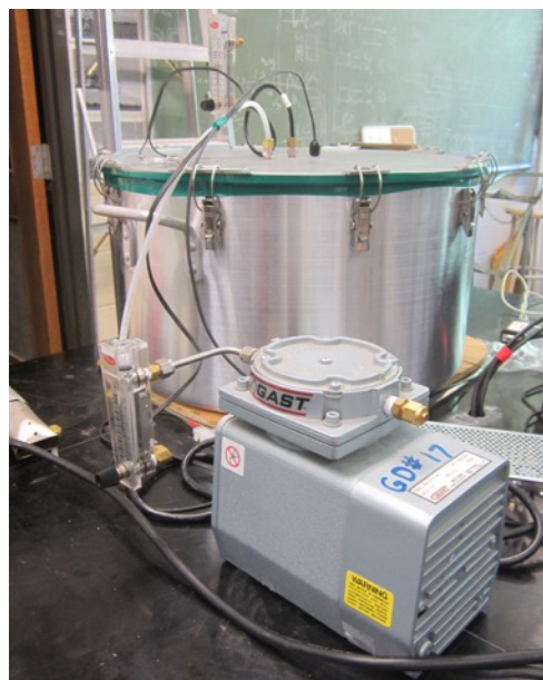
Figure 6 - Vacuum pump to evacuate the container.
