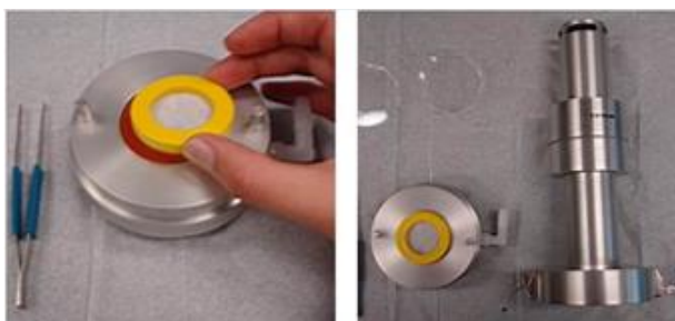
Figure 2 – Proper placement of filter into Harvard Impactor
