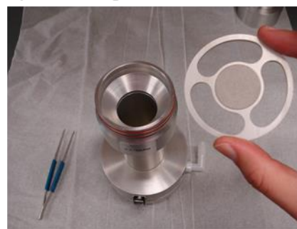
Figure 5: Installation of a clean and oiled impaction plate.
