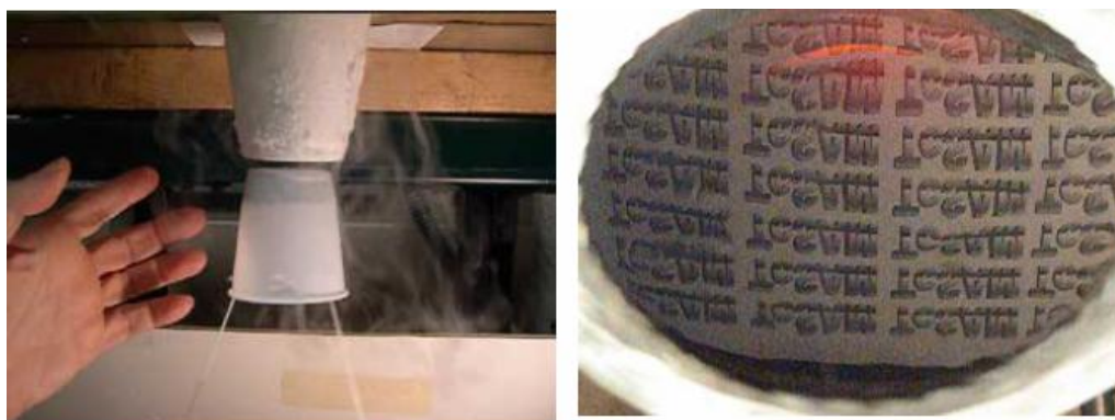
Fig 4. Model of spinning liquid mirror on a superconducting bearing by Ki Bui Ma, University of Houston. (a) shows the bearing, with a nitrogen-cooled YBCO superconductor in the upper cup, and a neodymium magnet in the inverted cup below. The gap is ~ 3 mm. Hanging on 3 strings below is a 20 cm spinning dish of black soy sauce with ~ 8" focal length (b). The lettering is the reflection of a screen above
