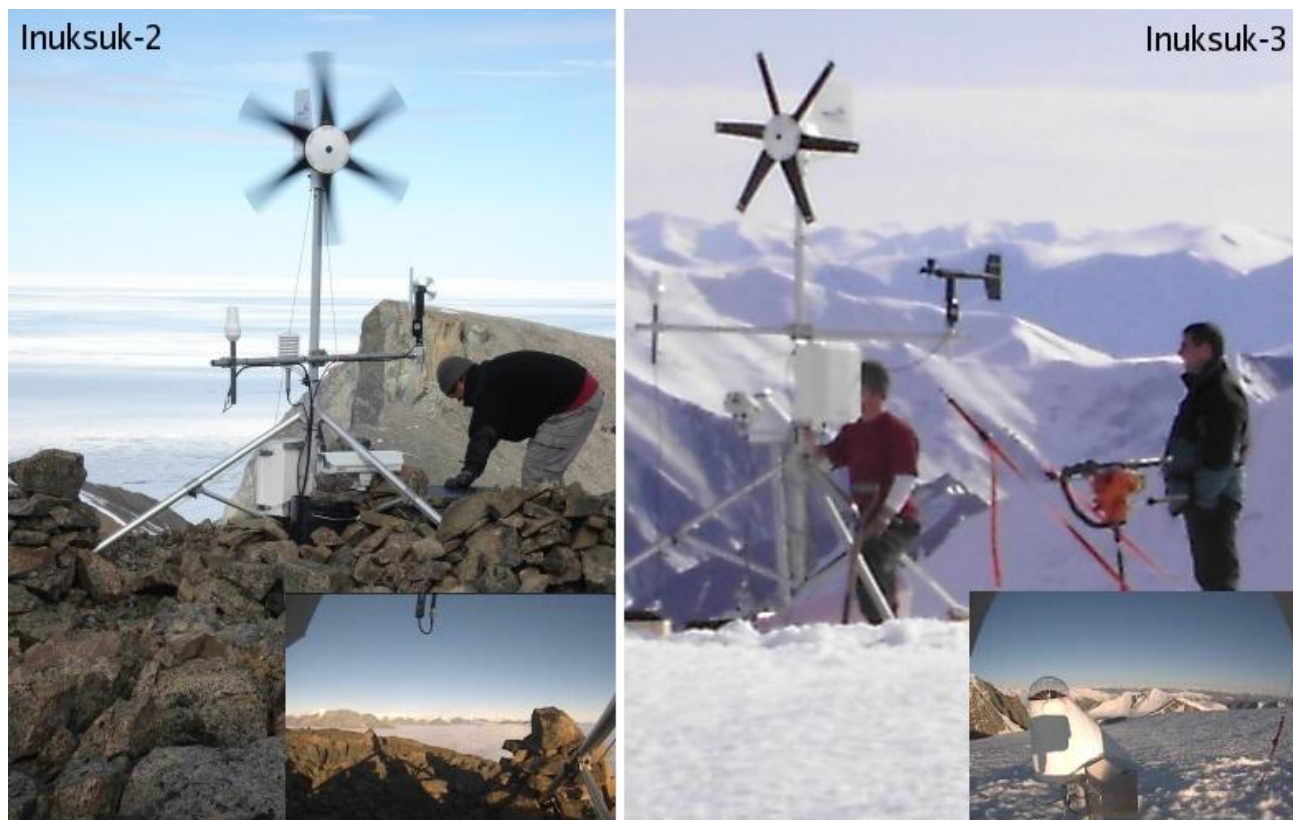
Figure 2 – Installation of a station on rock (left) and on snow (right). The piles of rock, and the general shape of the station led to the nickname “inuksuk” (plural “inuksuit” in the local Inuktitut dialect) like the stone way-markers common in Canada's high Arctic. Inset are images taken by each station's wide-angle “horizon camera.” The instrument visible in the centre of the Inuksuk-3 field of view is an all-sky camera.
