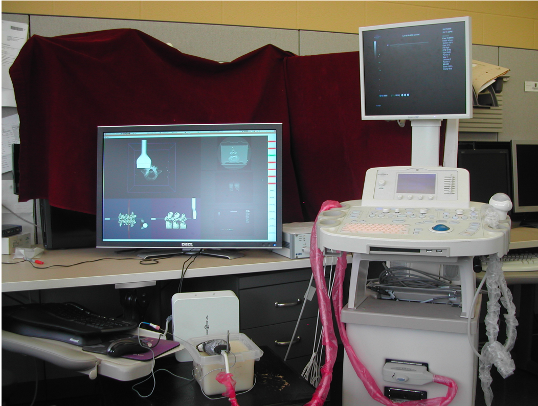
Figure 3. Apparatus of the spine-needle navigation system. The live US images are digitally acquired and displayed on the computer monitor.
