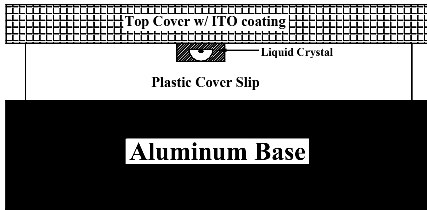
Fig. 6. Cross section of fabricated sensor
