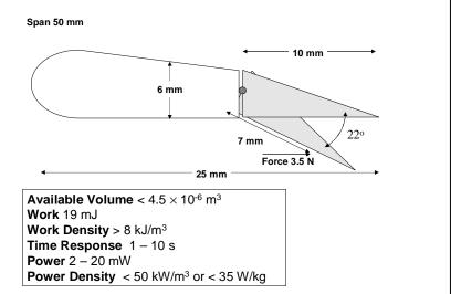
**Figure 1**: Blade Geometry. A cross-sectional view of a single propeller blade is shown, indicating the geometrical changes, forces and work needed to effect variable camber. The leading section (portion to the left of the pivot point) is assumed to have free volume available within.
