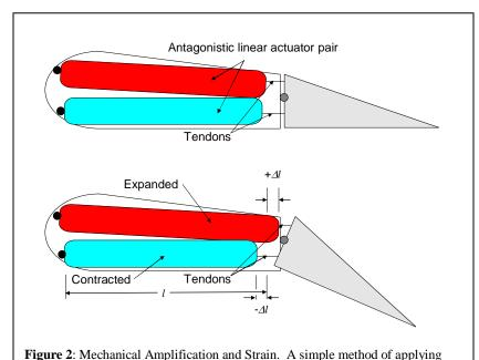
linear actuators to deflect the trailing edge of a foil is depicted above. Given the required deflections, the actuator strains must be approximately 25 %. (The image is not drawn to scale.) Smaller actuator strains will require amplification.
