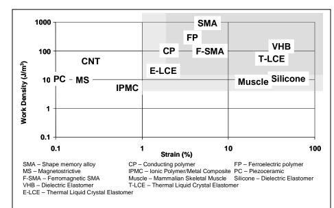
Figure 3: Plot of the approximate work densities and strains obtained in a range of actuator materials. In the variable camber application work density must be at least  $8 \text{ kJ/m}^3$ , and the optimal strain is approximately 25 %. The grey squares enclose candidate actuators. The work densities shown can be substantially higher than those achieved in practice, as discussed in the text.
