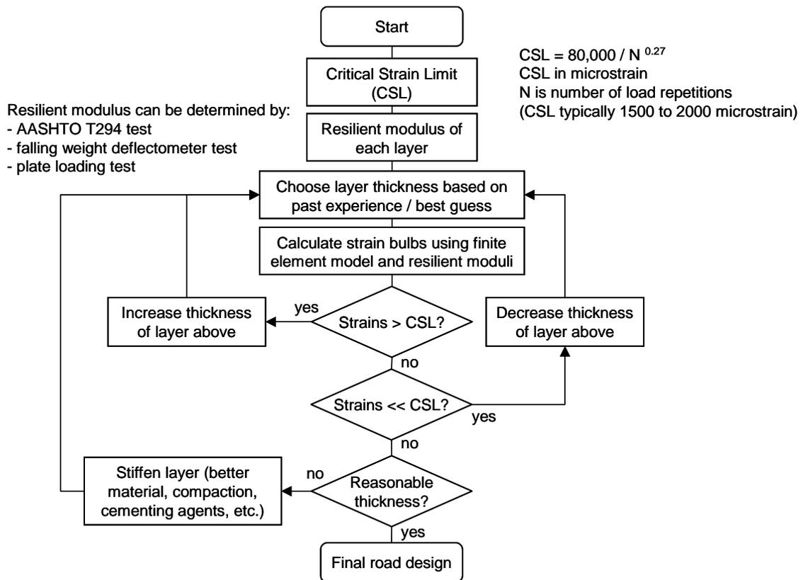
Figure 3-8 Major steps of the resilient modulus haul road design method.
