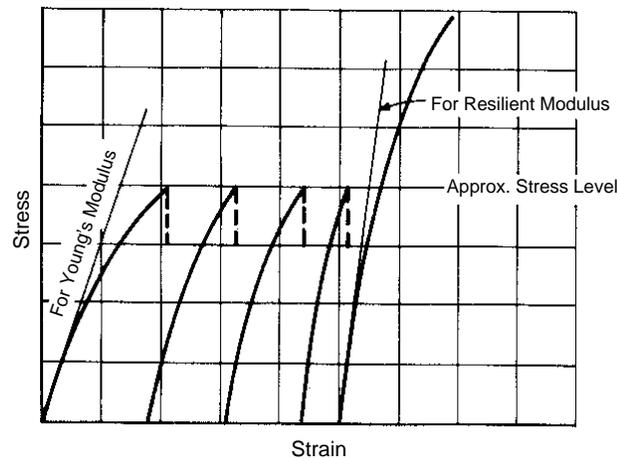
Figure 3-6 Method to obtain resilient modulus (after Bowles 1984).
