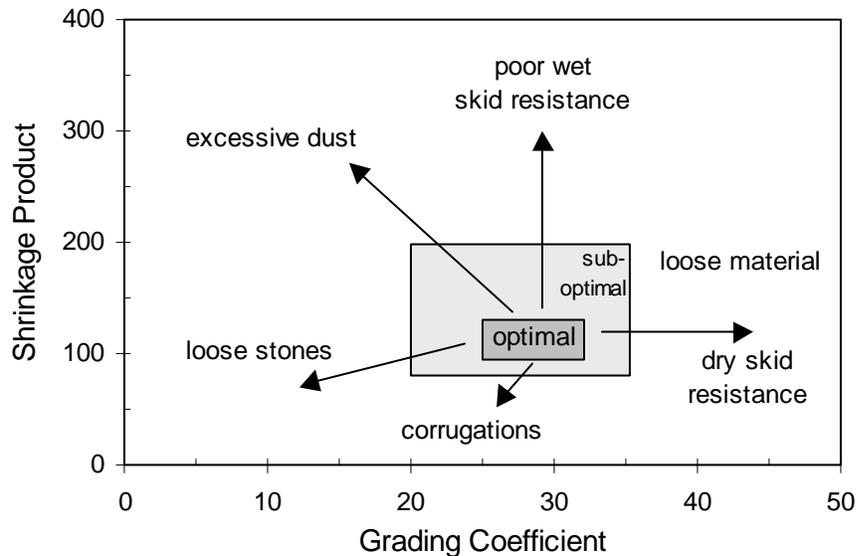
Figure 5-1 Optimal and sub-optimal range of values for the shrinkage product and grading coefficient for materials used on the road surface.
