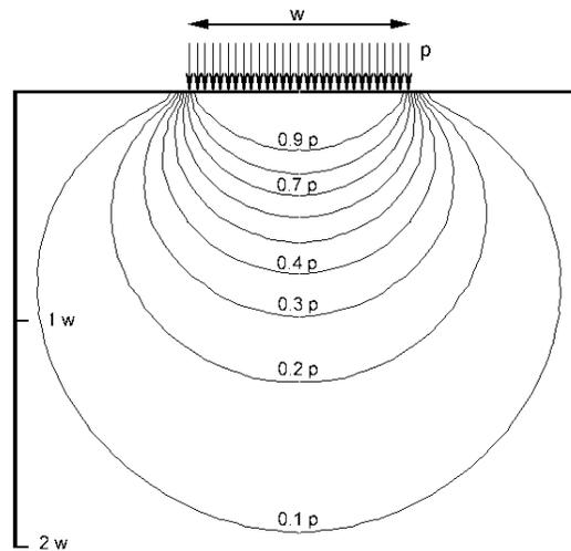
Figure 3-7 Stress bulbs below a circular pressure distribution.
