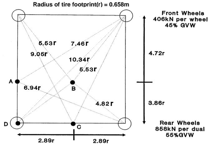
(b) Horizontal positions for critical points A B C D for R170 truck (fully laden)
