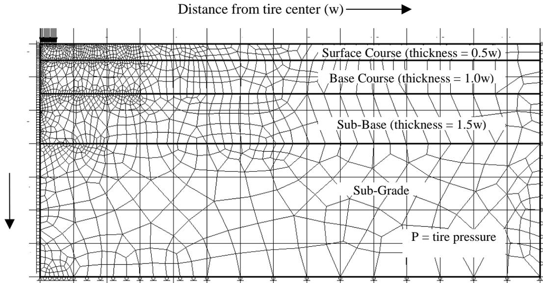
Figure 9-5 Axisymmetric model for case B study.
