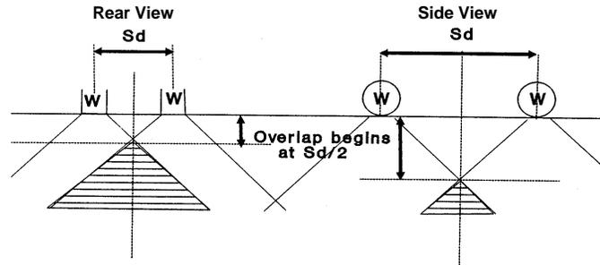
(a) Influence of multiple wheels on sub-grade stress for dual and front and rear axles
