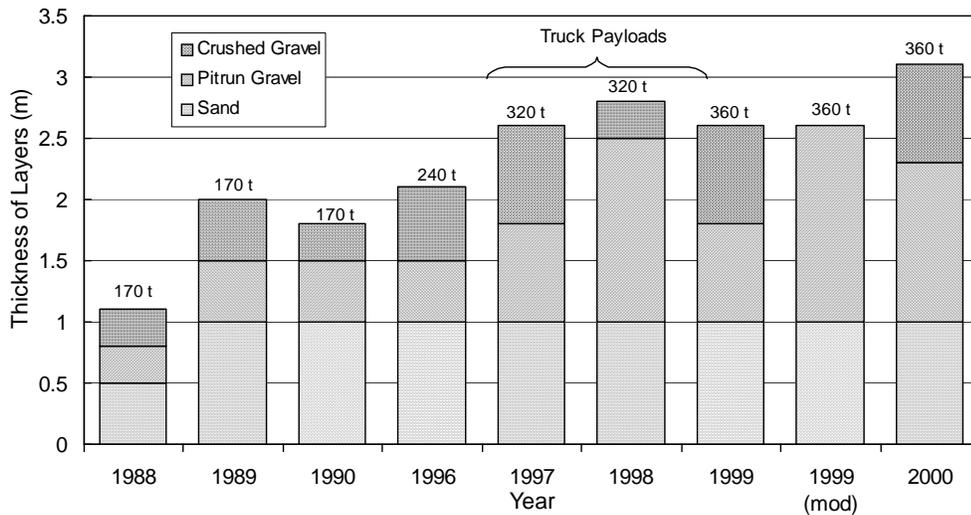
Figure 1-1 Change of haul road layer thicknesses with introduction of larger haul trucks.
