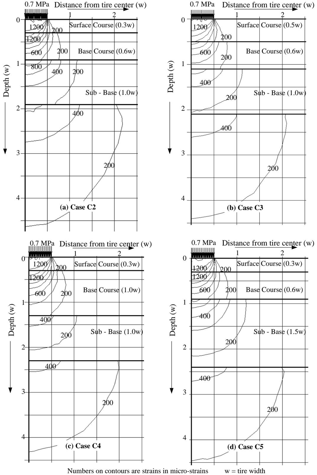
Figure 9-8 Vertical strain bulbs for different layer thickness.
