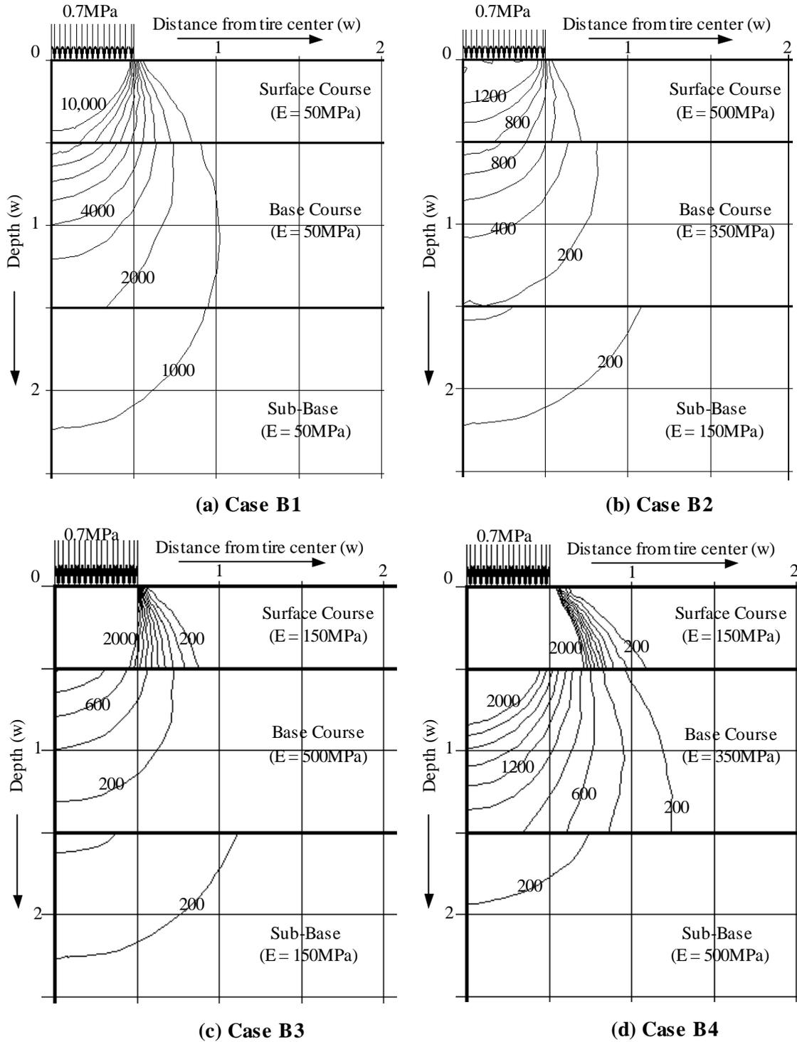
Numbers on contour are strains in micro-strain
