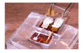
**Figure 2** Electroplating setup for the AgCl reference electrodes.
