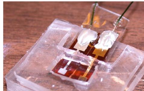
**Figure 3** The PDMS polymer enclosure around the flexible pH sensor.
