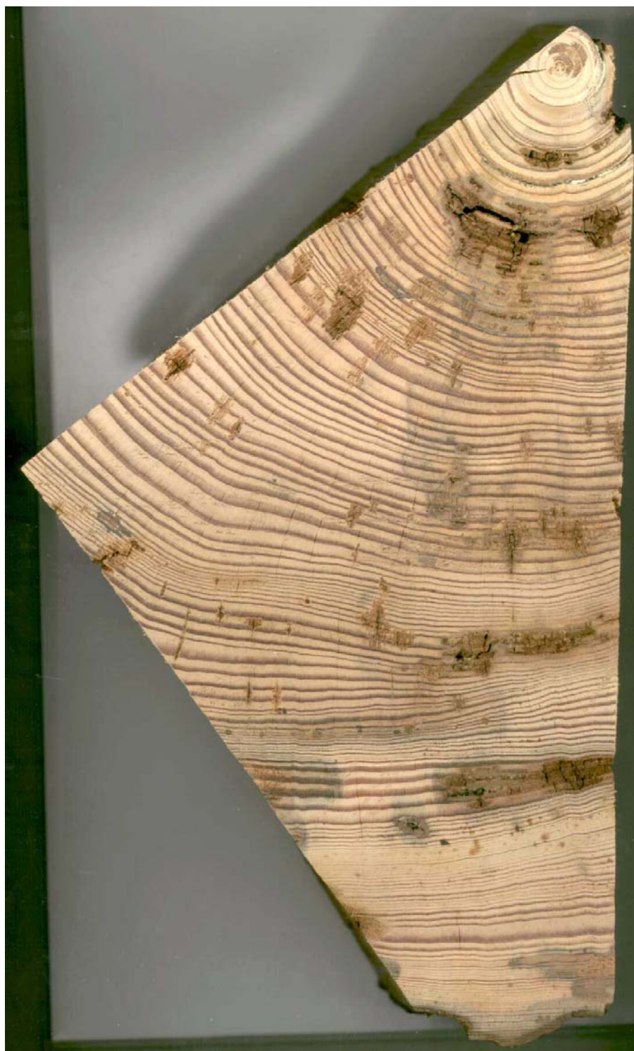
Figure 11. Sanded 'cookie' sample from Douglas fir stump used for the dendrochronological dating of F508.
