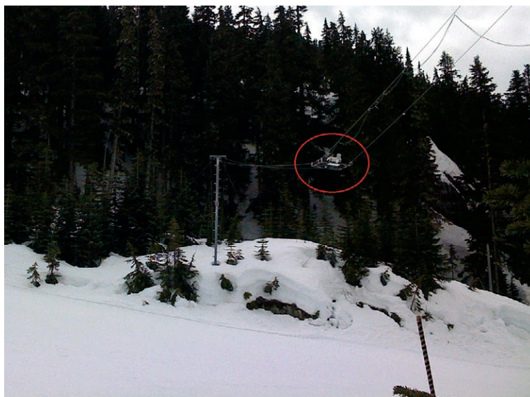
FIG. 5. Photograph at the Whistler RC IOP site showing the CNRI instrument platform (circled) and local trees that cause intermittent shading of a point below the instrument platform on a clear-sky day. The photographer is looking south-southeast across the piste (photo credit: Rosie Howard).
