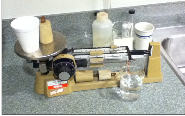
Figure 1: Experimental Setup. From left to right, the Styrofoam cup for addition of water as mass applied, calibration bulk weight of 1 kg, minor control knob to obtain equilibrium position, three beams (two are used for balancing and the third for the attachment of ring), and the ring for contacting the periphery of the fluid.
