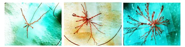
Figure 2. False-colour photographs of aggregates grown at 8V, 12V and 16V respectively.
