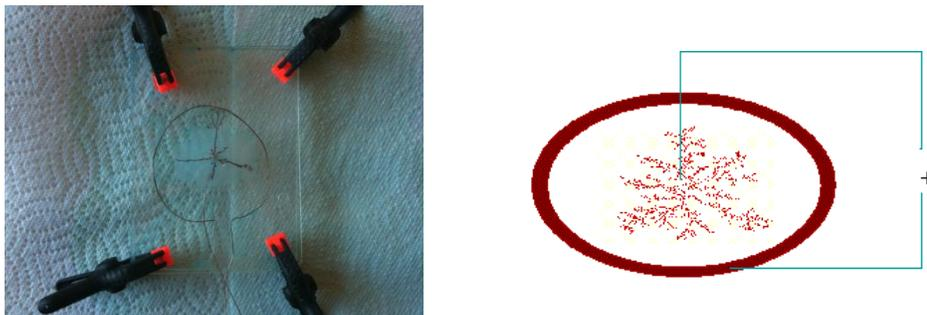
Figure 1. *Photograph and schematic of electrolytic cell, showing cathode and anode wires, along with a small aggregate. Schematic reproduced without permission from [4].*
