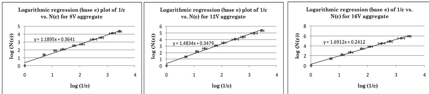
Figure 3. Graphed box-counting data from the aggregates in the previous figure, showing respective dimensions of 1.19, 1.48 and 1.69. Vertical error bars in  $N(\epsilon)$  too small to be visible.
