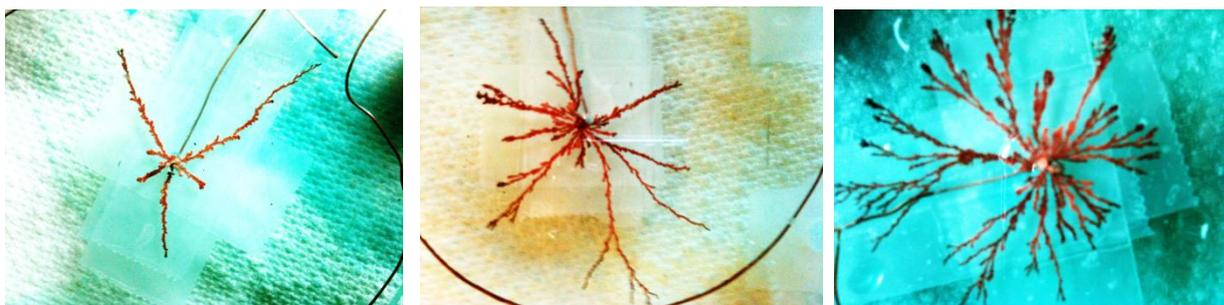
**Figure 2.** *False-colour photographs of aggregates grown at 8V, 12V and 16V respectively.*
