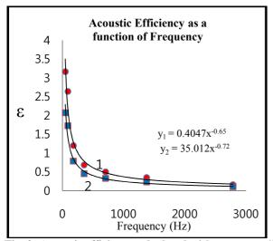
Fig. 2: Acoustic efficiency calculated with respect to 1) surface area of the room; 2) inverse square model  $(4\pi r^2, r=6m)$ . The region between the two fits is where the true acoustic efficiency value is likely to be found in. Error bars were avoided as the largest uncertainty estimate was around a factor of 3 considering figure 4.
