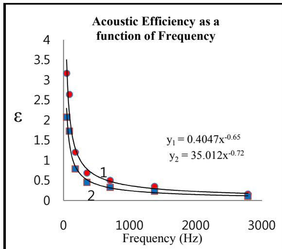
**Fig. 2:** Acoustic efficiency calculated with respect to 1) surface area of the room; 2) inverse square model ( $4\pi r^2$ ,  $r=6m$ ). The region between the two fits is where the true acoustic efficiency value is likely to be found in. Error bars were avoided as the largest uncertainty estimate was around a factor of 3 considering figure 4.
