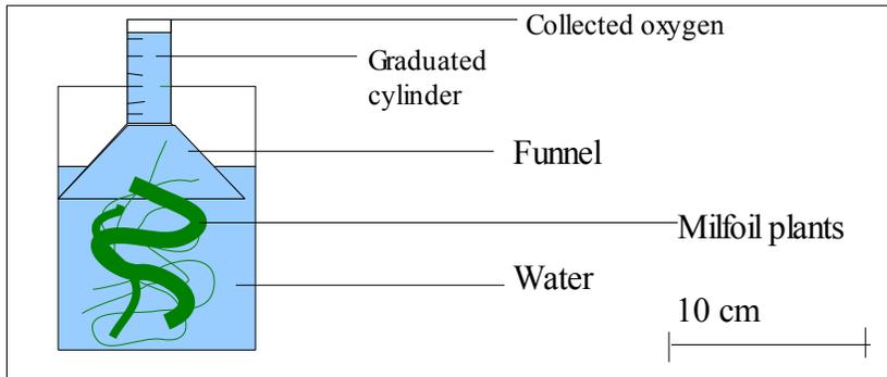
Fig. 1 Apparatus used for collecting oxygen during photosynthesis.
