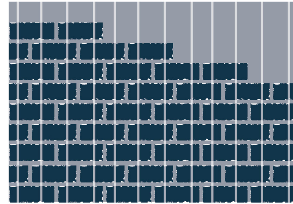
Fig 26. Salvaged Bricks with Infill to match new Brick Course Source: Author, 2022
