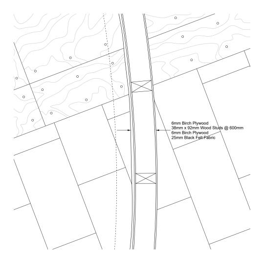
The lights are placed on top of installation along with a carefully curated opening. I designed the openings to control the light and contain it within the volume and placed them away from the wall surface to reduce the bouncing of light. A reveal along with a cover continues along the wall to allow the flow of air and dust but block any exterior light.
