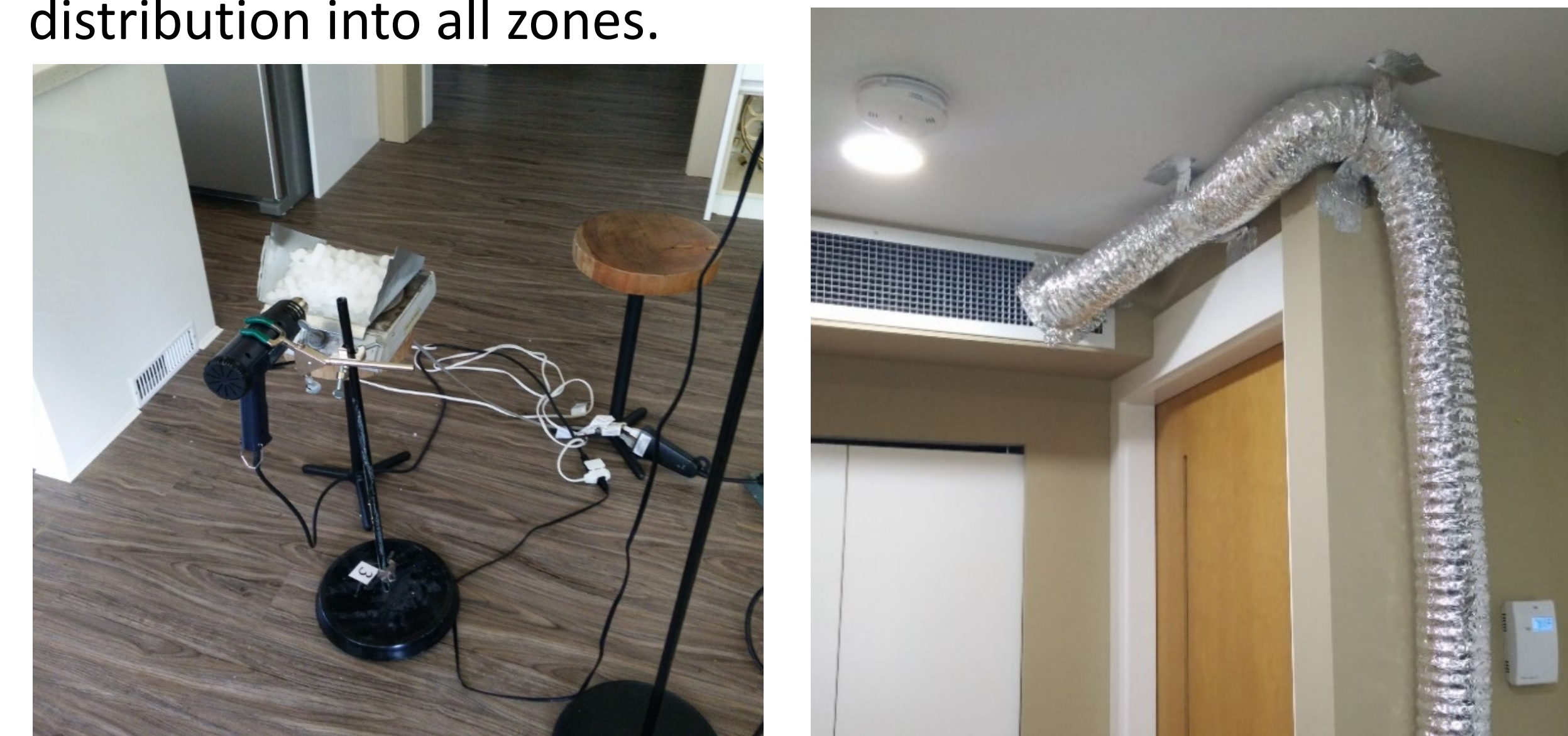
Tracer gas tests experimental setup at the AYO house
