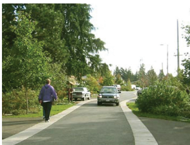
“Flat curbs” visually narrow the width of the roadway, which slows traffic (Seattle Public Utilities, 2003).
