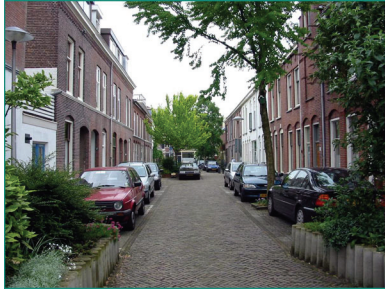
A woonerf uses a variety of paving materials to designate space and use like this one in Delft.
