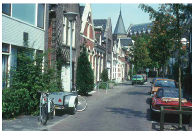
Woonerven realign the roadway to slow traffic and provide parking and play space. This woonerf provides bike racks, too.
