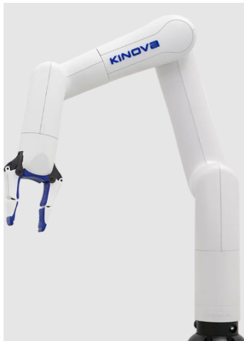
Figure 2.1: Kinova Gen3 Lite manipulator 1
