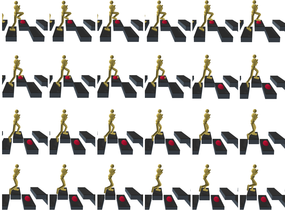
Figure 6.5: 24 consecutive environment control steps at 60 Hz (16.7 ms between frames) for the humanoid stepping stone task. Each row corresponds to one chunk of actions using an H = 6 chunk-only policy, lasting 100ms.
