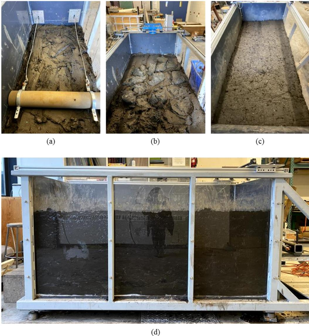
**Figure 4.15 Photographs showing the process of test soil bed preparation after pipe placement: (a) Connecting the pipe and pulling cables; (b) Placing the soil cover in loose lifts of 6-8 inches; (c) Plan view of the SPI test chamber prior to a horizontal pipe displacement test; and (d) Side view of the SPI test chamber prior to a horizontal pipe displacement test**
