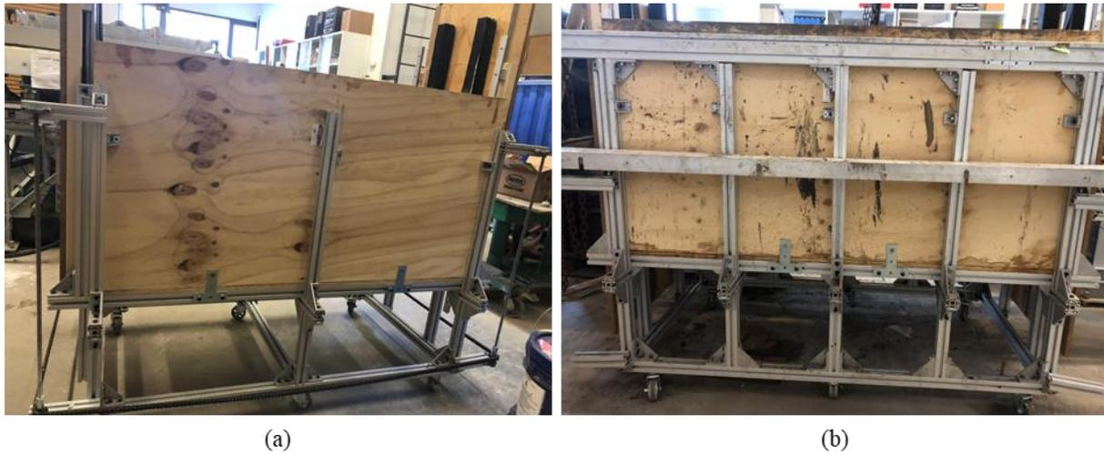
**Figure 4.2** Photographs taken (a) before and (b) after installation of the aluminum structure to reinforce the axial SPI test chamber
