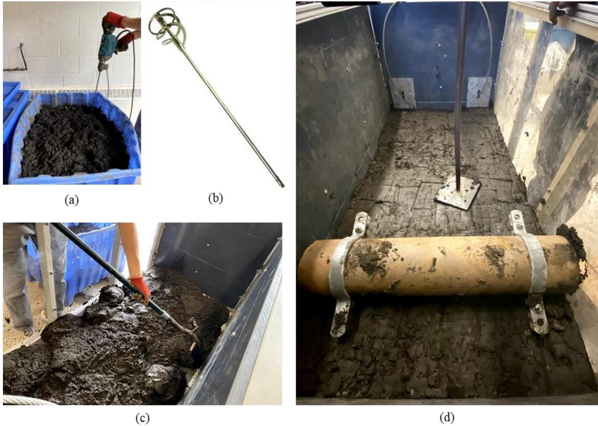
**Figure 4.14** Photographs showing the process of test soil bed preparation prior to pipe placement: (a) Mixing of organic soil to achieve a relatively uniform soil mix; (b) Soil mixer paddle; (c) Placing the soil in loose lifts of 6-8 inches prior to leveling; and (d) Pipe placement on the prepared soil bed (dense) before placing the soil cover
