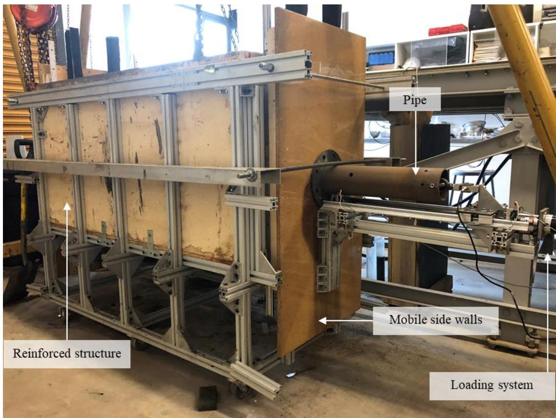
Figure 4.1 Perspective view of the axial soil-pipe interaction test apparatus
