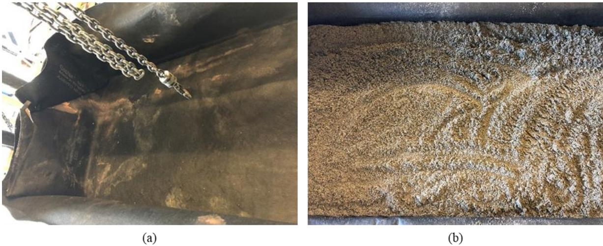
**Figure 4.8 a) Placement of geotextile on prepared organic soil cover; and b) Preparation of FR sand bed in layers**
