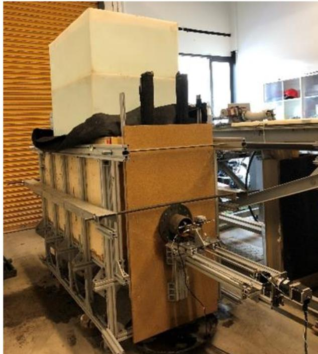
**Figure 4.9** Final set up of the SPI test chamber prior to axial displacement test
