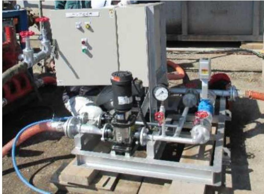
**Figure 3-5 Temperature control unit.**
