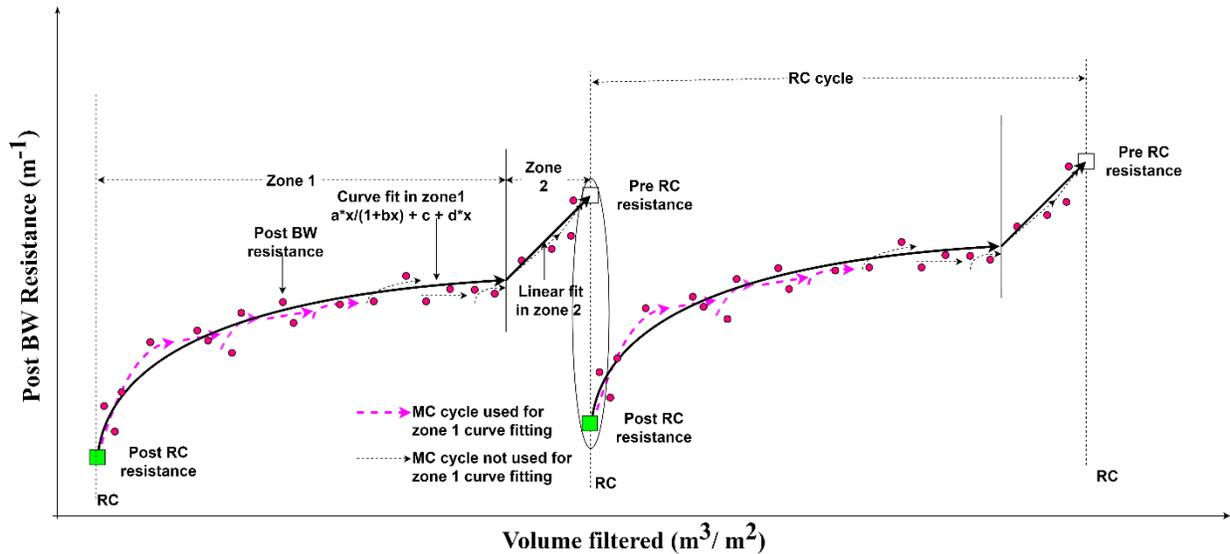
Figure 3: Change in post BW resistance between RC
