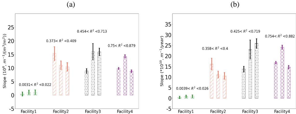
Figure 7: Rate of change of estimated clean membrane resistance
