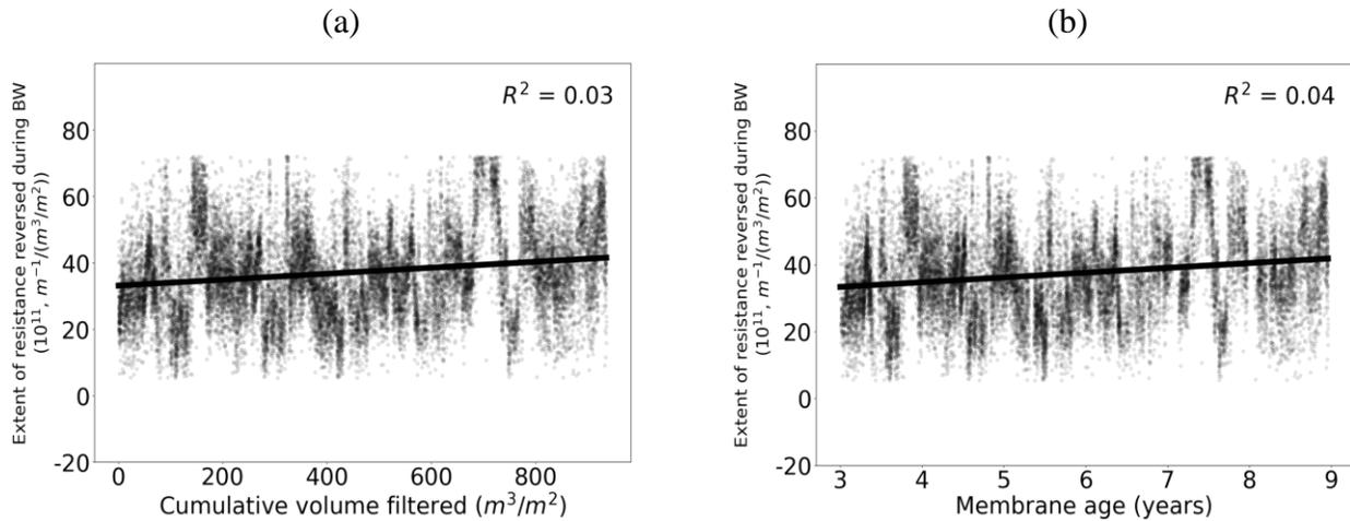
Figure 10: Typical extent of resistance reversed during BW
