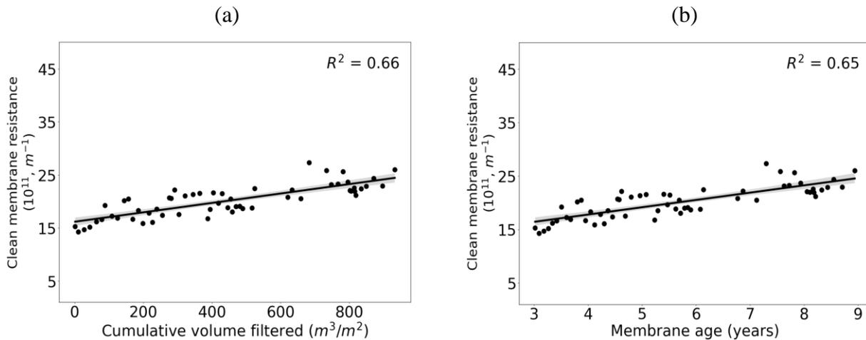
Figure 6: Typical clean membrane resistance
