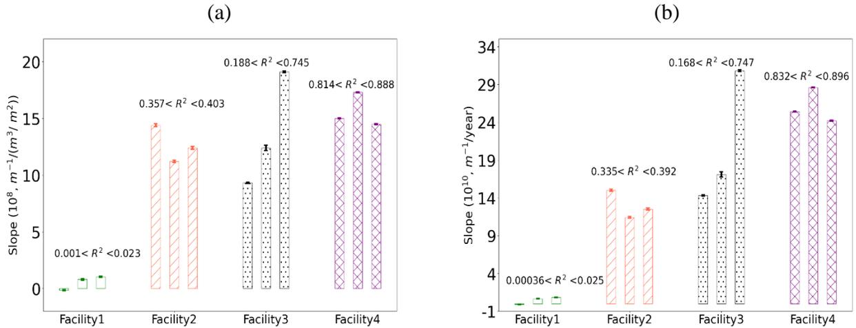
Figure 5: Rate of change of estimated hydraulically irreversible resistance
