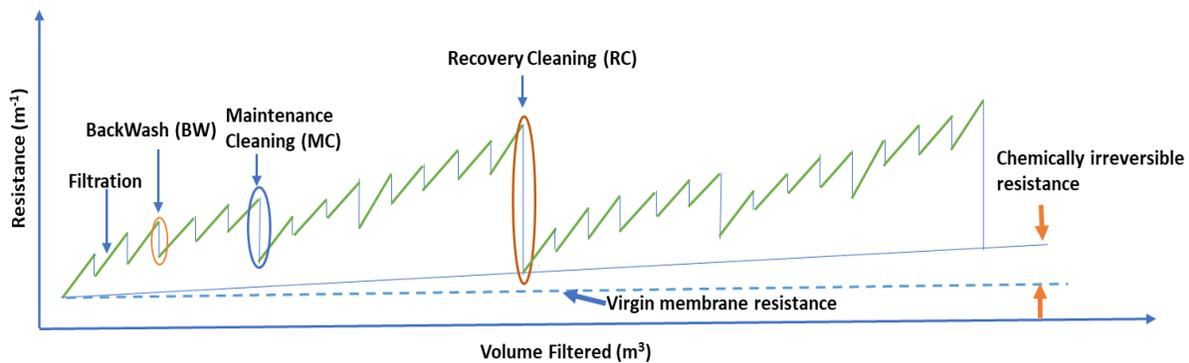
Figure 1: Resistance evolution in membrane during filtration and cleaning
