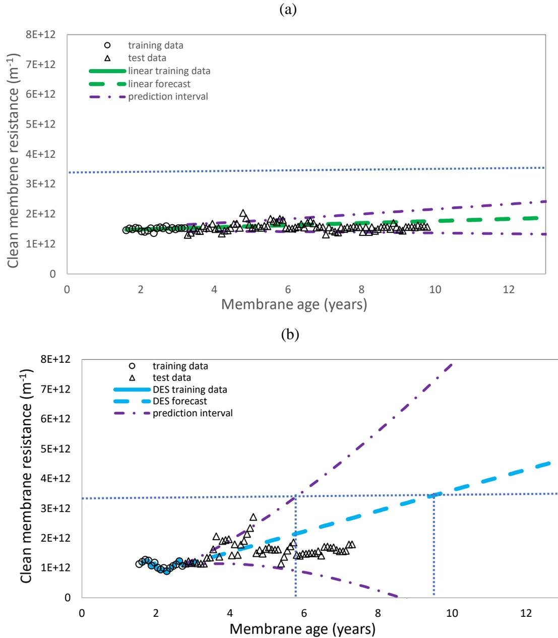
Figure 16: Forecasting membrane replacement
