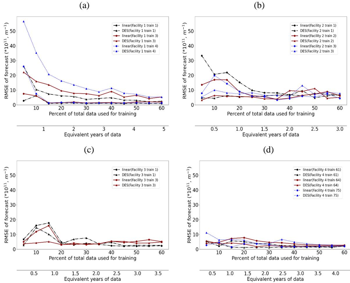
Figure 15: RMSE of the test data between forecasted and actual clean membrane resistance.
