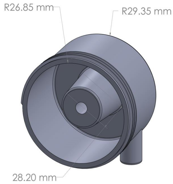
Figure A3: Active cyclone lid geometry and dimensions.
