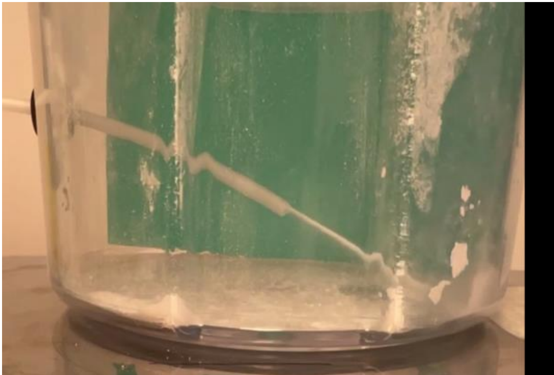
Figure 10: Particles flow at the outlet of the catheter at a 0.37 \text{ m}^3/\text{h} air flow rate during experiments.
