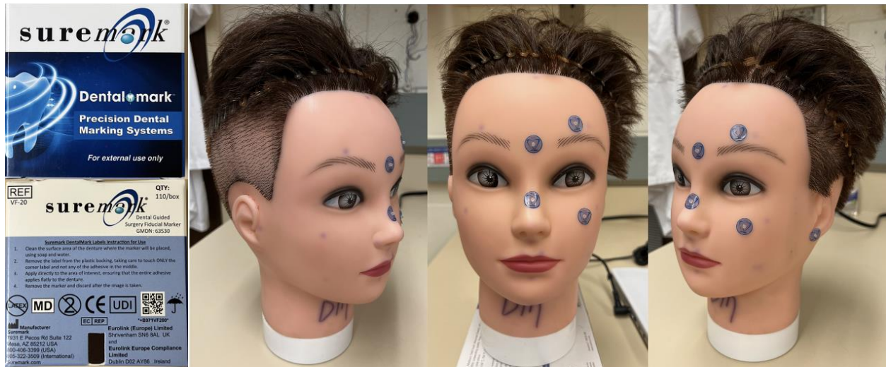
Figure 2.4: Placement of the Five Suremark Fiducial Markers
