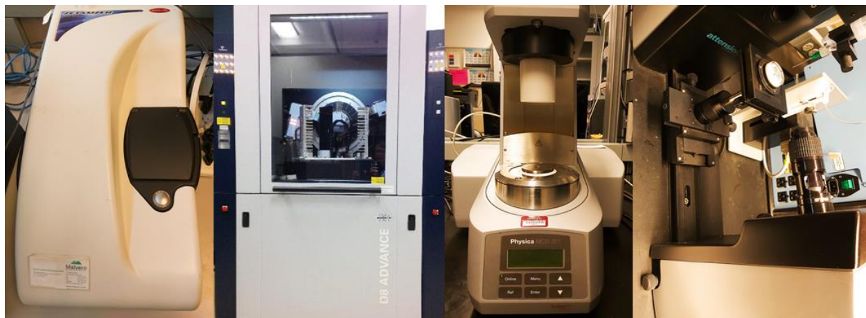
Fig. 3.5: (from left to right) Malvern Zetasizer Nano ZS for dynamic light scattering measurements, Bruker D8 Advance x-ray diffractometer, Anton-Paar Physica MCR 301 rheometer and Biolin Scientific Attension Theta tensiometer.
