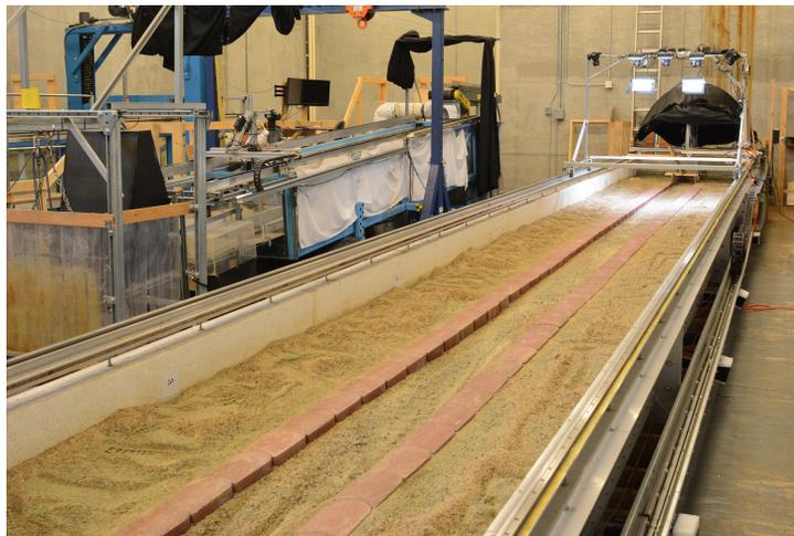
Figure 3.1: Adjustable-Boundary Experimental System (A-BES) at the University of British Columbia, featuring cameras (top-right) and bank control system at a width of 30 cm.
