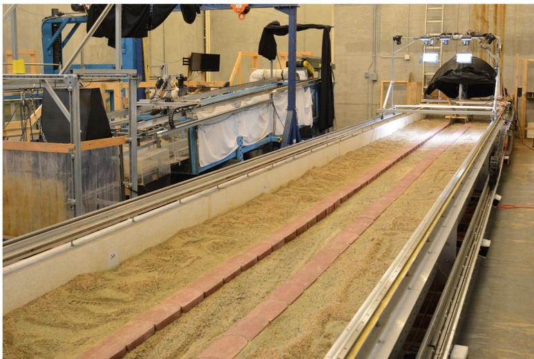
**FIGURE 1** Adjustable-boundary experimental system (A-BES) at the University of British Columbia, showing the 30 cm channel configuration (Adams & Zampiron, 2020, CC BY 4.0)
