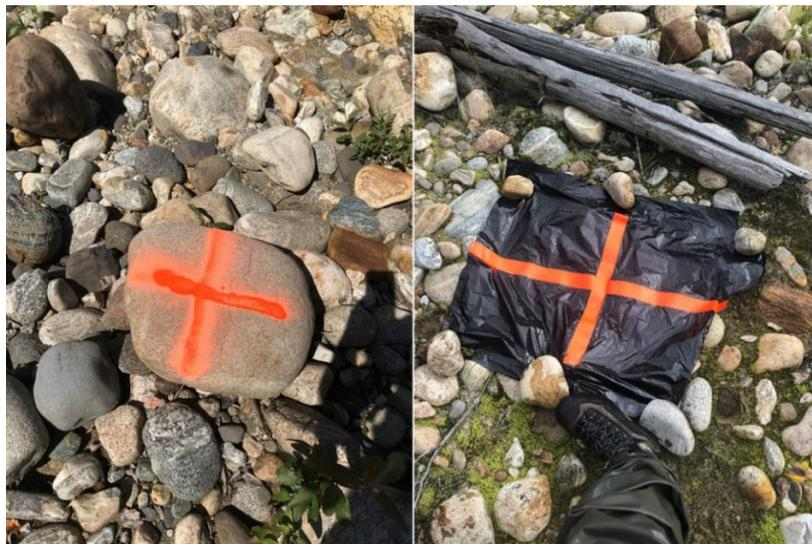
*Figure 3.8 Examples of ground control markers deployed in the field, including the initial test markers (left) used for the July 25h and Aug. 14th test flight, as well as the high contrast markers (right) employed on the final Sept. 30th flight.*
