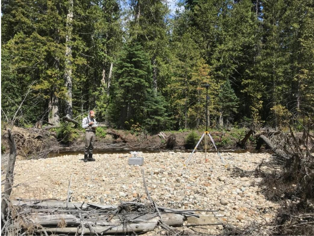
Figure 3.7 Ground level photo of the RTK -DGPS base station and drone lunch pad, at the gravel bar mid-reach, between transects 14-16 (August 13th, 2019).
