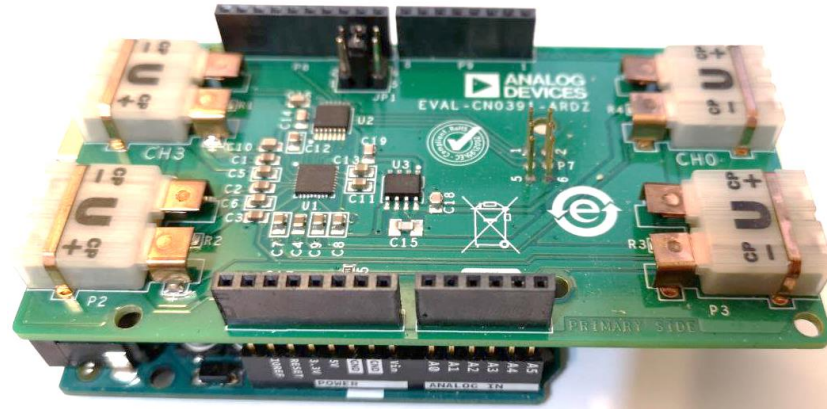
Figure A.5. Thermocouple module mounted on Arduino Uno board.
