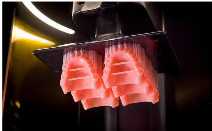
**Figure 4: 3D Printed dentures using SLA technology**
