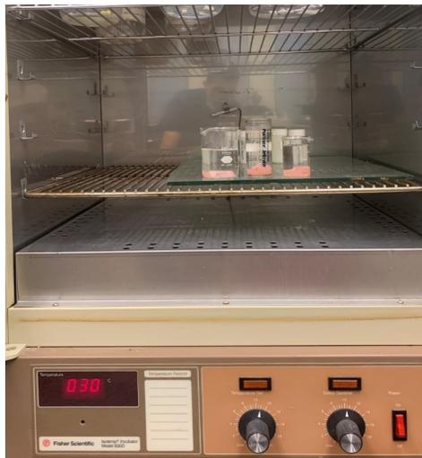
**Figure 14: Samples being aged in an Incubator**
