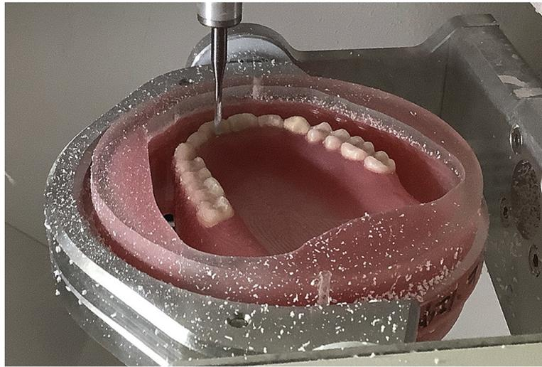
**Figure 3: CAD/Milled Denture Base Processing (51)**
