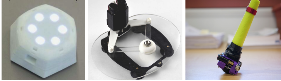
Figure 5.2: Three educational haptic devices used in this work. From left to right: Cellulo [171], Haply [67], and MagicPen[113].
