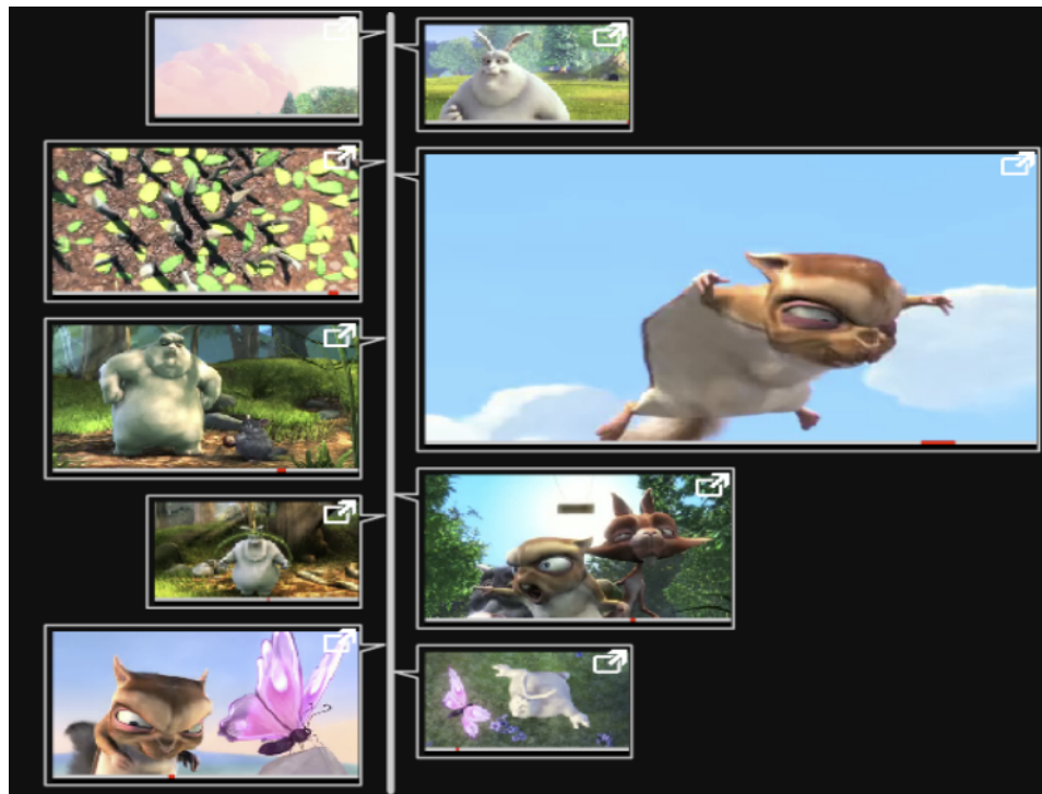
Figure A.1: The video timeline is a visualisation of intervals of video that users have watched previously. The timeline is generated dynamically from the user's searching behaviour; larger thumbnails represent intervals that have been visited more often. (Al Hajri et al. [5]) Video thumbnails © copyright 2008, Blender Foundation / www.bigbuckbunny.org . Used with permission.
