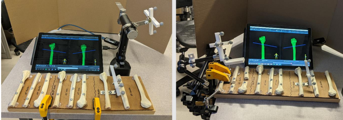
Figure 55 - OTS (left) and OTG (right) cut guidance method set up
