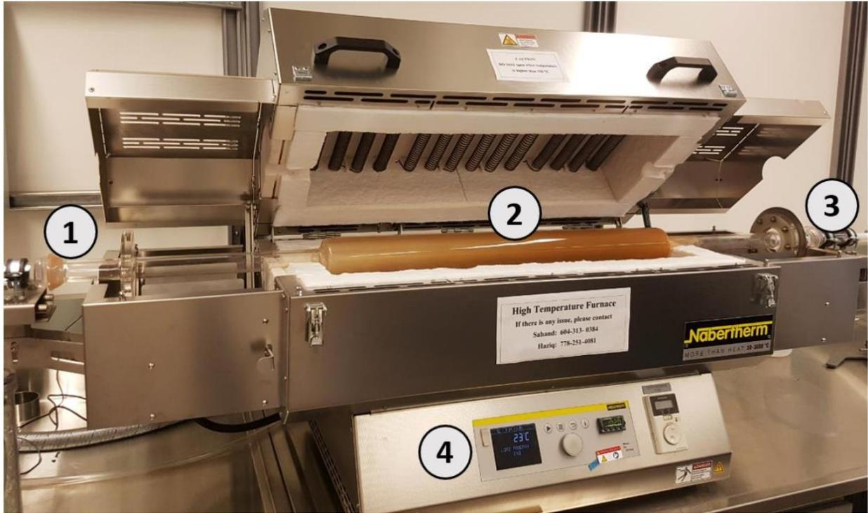
Figure 4.4 Horizontal tube furnace including (1) gas inlet, (2) quartz tube, (3) gas outlet, and (4) temperature controller.
