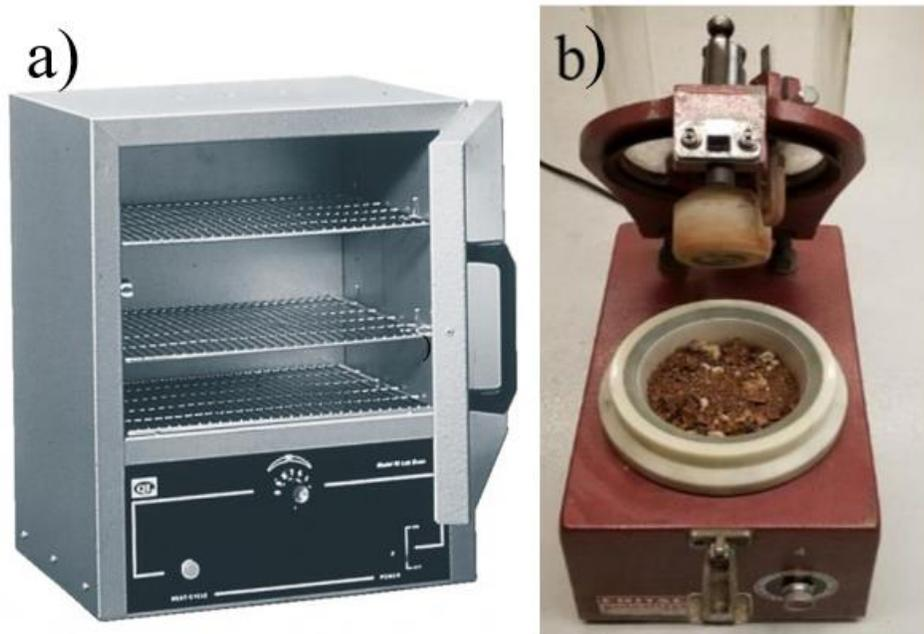
Figure 4.2 (a) Oven, (b) mortar grinder mill.
