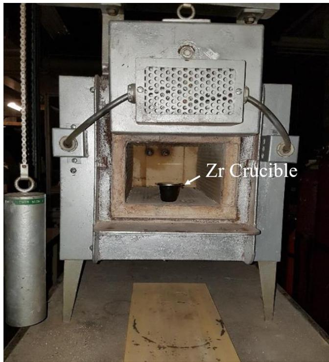
Figure 4.9 Muffle furnace.
