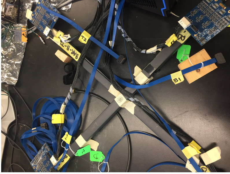
Figure 7.11: Crossed bar layout for the vertical slice. In this layout, coincidence events are localized to the overlap of the two bars.
