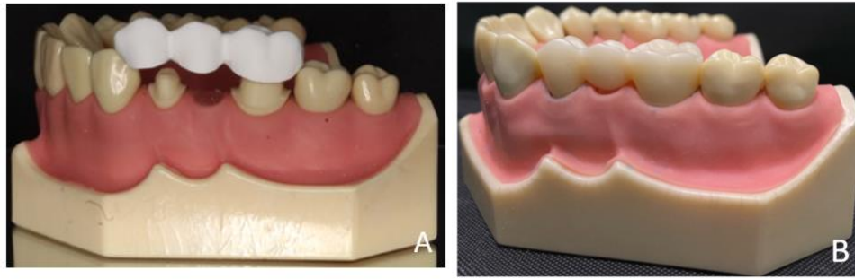
Figure 4. The difference in the size of the monolithic zirconia before and after fast-sintering: A. Milled monolithic zirconia 3-unit FDP before fast-sintering. B. 25% shrinkage of the monolithic zirconia 3-unit FDP after fast-sintering.
