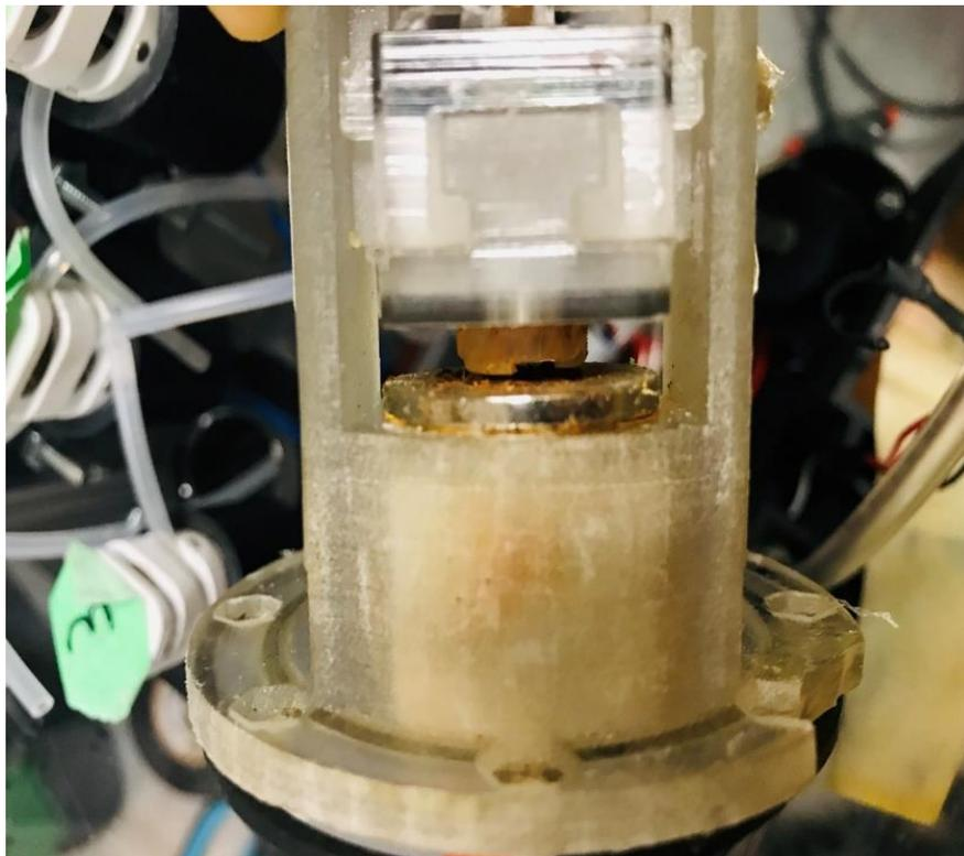
*Figure 2.10 Corroded magnet in Version 1.*
