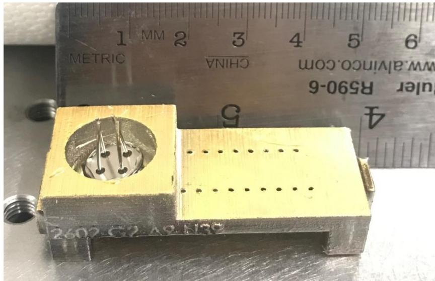
*Figure 2.1 The Selective microfluidic system embedded with a MOS sensor*
