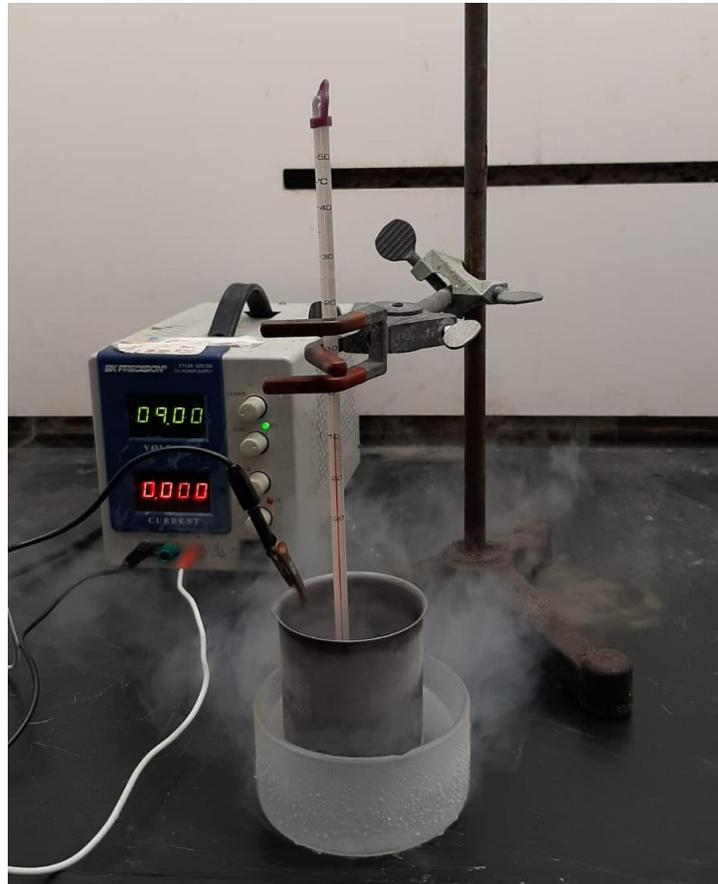
**Figure 4.12: Setup used for electro-etching**
