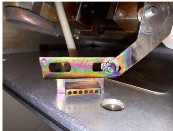
Figure 4.8: Quench head used in the Gleeble heat treatment
