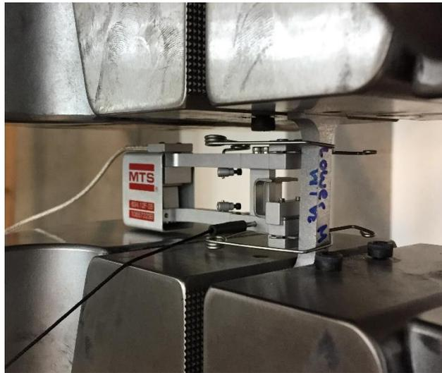
Figure 3.5-1. Tensile test setup including MTS extensometer
