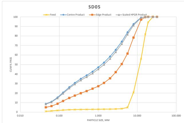
**Figure A.40: Feed and product PSDs of test Quarry SD-05**
