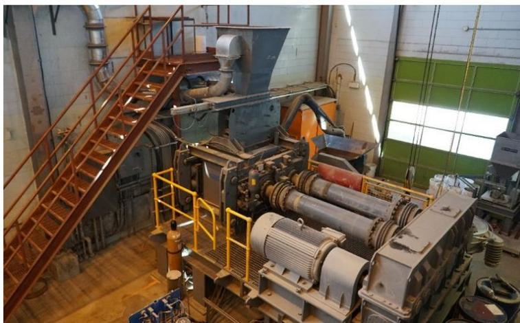
**Figure 3.2:** Pilot HPGR facility at UBC
