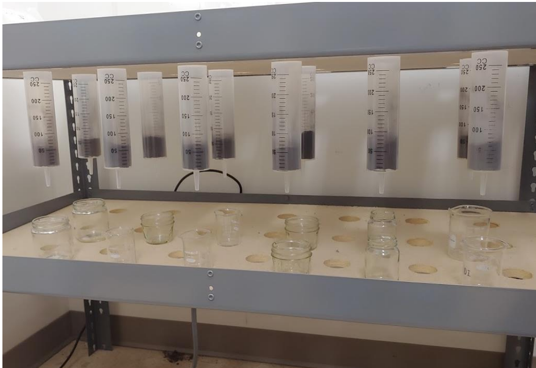
Figure 11: Soil and K_3PO_4 samples packed into PVC syringes
