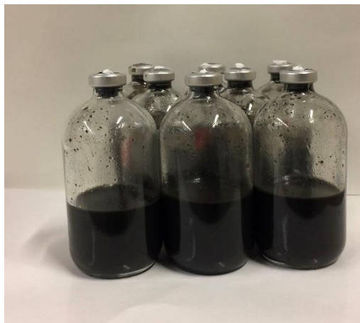
Figure 3-5. Biochemical methane potential (BMP) assays using serum bottles (160 mL)
