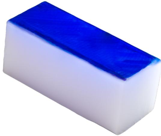
**Figure 3.3:** 22mm length prepared Delrin specimen, marked with blue marker for proper orientation.
