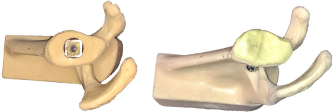
**Figure 3.6:** The uncovered drilling jig (left) and the glenoid surface covered with plasticine (right) in order to prevent the user from using visual cues related to the plastic insert and tube when choosing the drill entry point.
