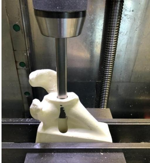
**Figure 3.1:** SAWBONES scapula bone model in the midst of preparation to be used as our surgical jig.
