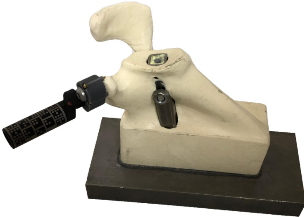
**Figure 3.2:** Prepared bone model mounted onto a steel block. The steel tube insert is visible in the glenoid fossa at top.
