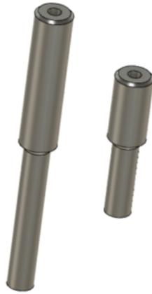
**Figure 3.4:** Custom made measuring pins with a stem machined to  $4.4\text{mm} \pm 0.1\text{mm}$ .
