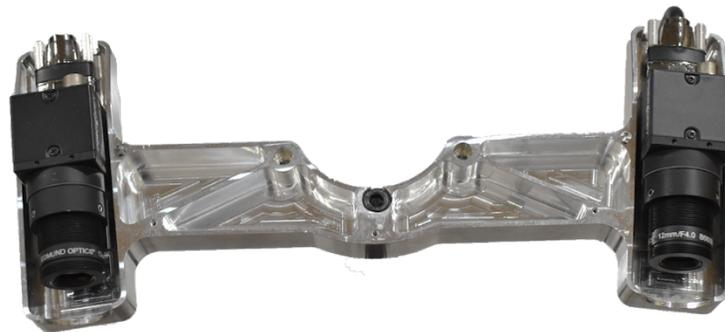
**Figure 2.16:** Point Grey FL3-U3-32S2M-CS cameras mounted onto the NST stereo camera mount made of a rigid aluminum construction, acting as both a heat sink and mechanical mount.
