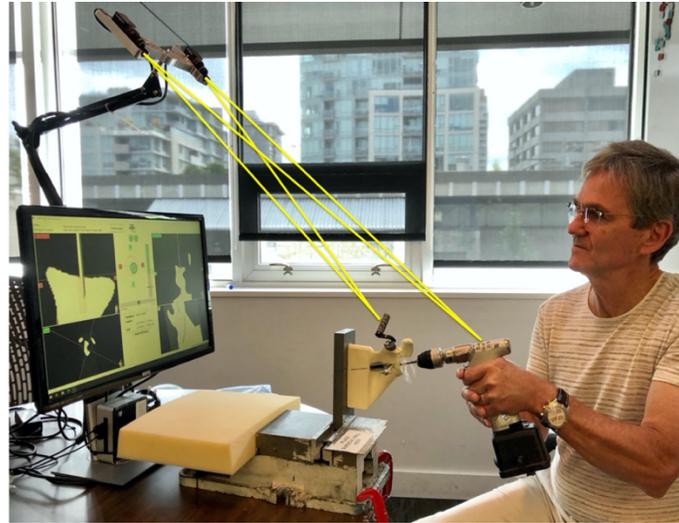
**Figure 3.5:** Surgical system setup on day of the mock trials, with the attending orthopaedic surgeon holding the drill. The cameras were mounted on the back of the monitor mount, looking down at the surgical drill and patient tracker. The drilling jig was mounted vertically on a vise which was clamped down to the table.
