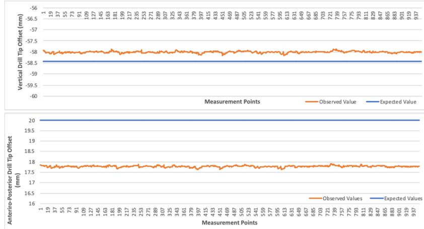
**Figure 4.3:** Superior-inferior (top) and anterior-posterior (bottom) offset of drill tip over 941 samples (orange), relative to a predefined point on the calibration phantom (blue).
